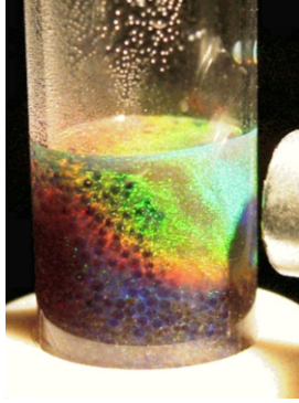
Figure 3. Magnetophoresis of cobalt ferrite/silica core-shell particles in the presence of a field gradient originating from the permanent magnet at the right-hand side. In the vicinity of the maximum field gradient, the lattice constant of the colloidal crystals decreases. As consequence, a shift of the backscattered light from red to blue colour can be observed. The dark spheres are ion exchanger resin.
